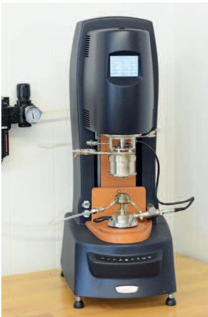
*TA Instruments DSC-25 Differential Scanning Calorimeter*
